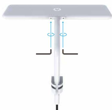
2 Adjust the height and tighten the screws
